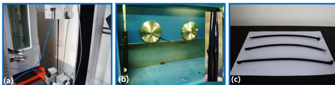
Figure 2. The measurements of (a) tensile loading, (b) burst pressure and (c) fuel permeability for the fuel pipes of automobiles.
