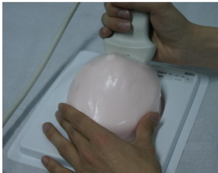
Figure 3 The tissue-mimicking breast phantom used in the phantom study. The acquisition of ultrasound RF data of the breast phantom with freehand scan.
