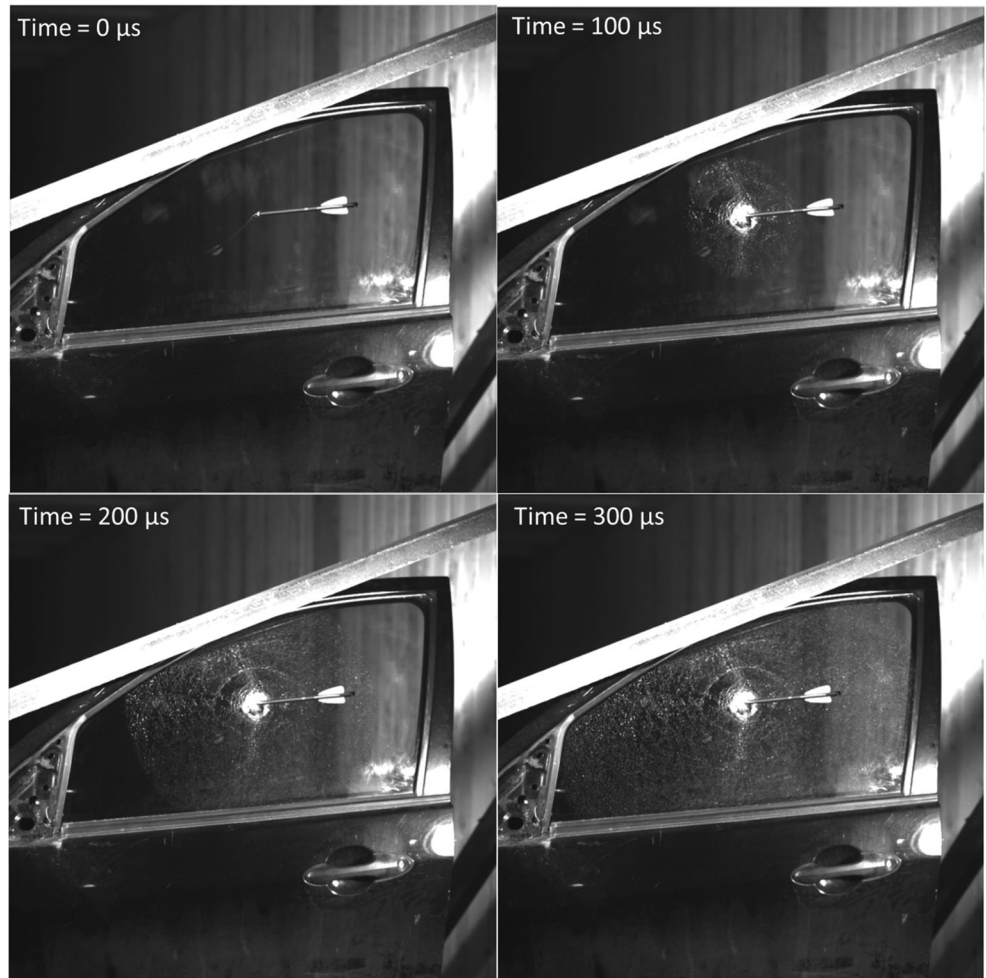
Fig. 7 Glass failure during impact with crossbow bolt between 0 to 300 \mu s during test 1
