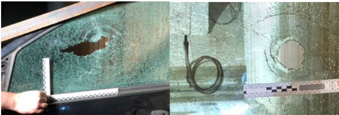
Fig. 6 Fracture pattern post impact by a 2219 bolt and EK Bolt in to window 1 and 6, respectively
