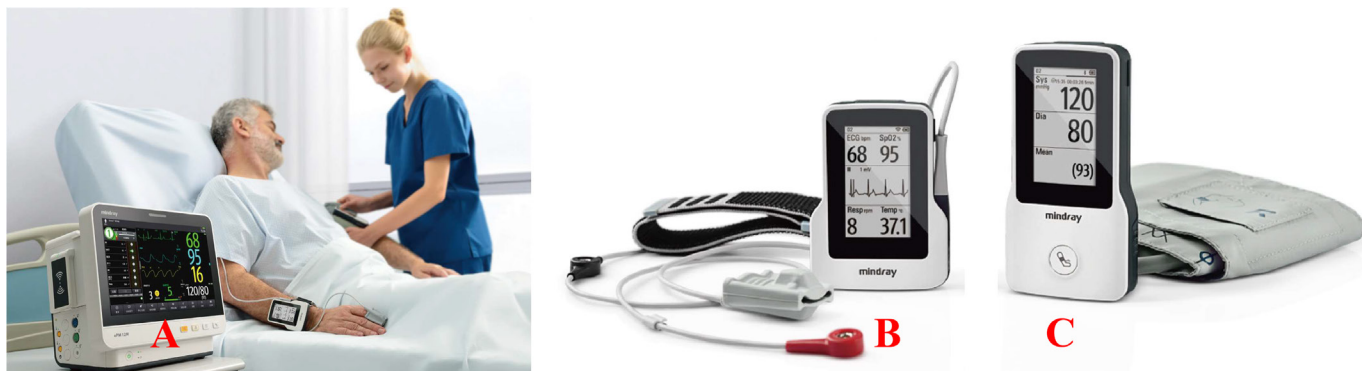
Figure 2 Simulated patient monitoring with the ePM/ep pod series monitor (includes a demonstration of a training). (A) The bedside component (ePM) displays the patient's vital signs, received wirelessly. (B). The ep pod can monitor three-lead electrocardiography output, SpO 2 , respiratory rate and daily ambulation duration. (C) The bp pod non-invasively records the patient's blood pressure. *Note: Mindray Medical International has authorised the copyright of the figure, in which the people depicted are not patient and were taken with the participants knowledge. The person in the demonstration of training is not our patients. SpO 2 , oxygen saturation.
