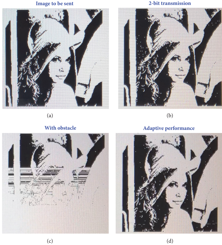
FIGURE 6: Measurement results of the DDM wireless communication system. (a) The original image to be transmitted. (b) The received image under the 2-bit-symbol transmission mode. (c) The received image when a metal plate is placed between the programmable metasurface and two receiving antennas. (d) The received image after running the channel autoscan program when a metal plate is placed between the programmable metasurface and the two receiving antennas.
