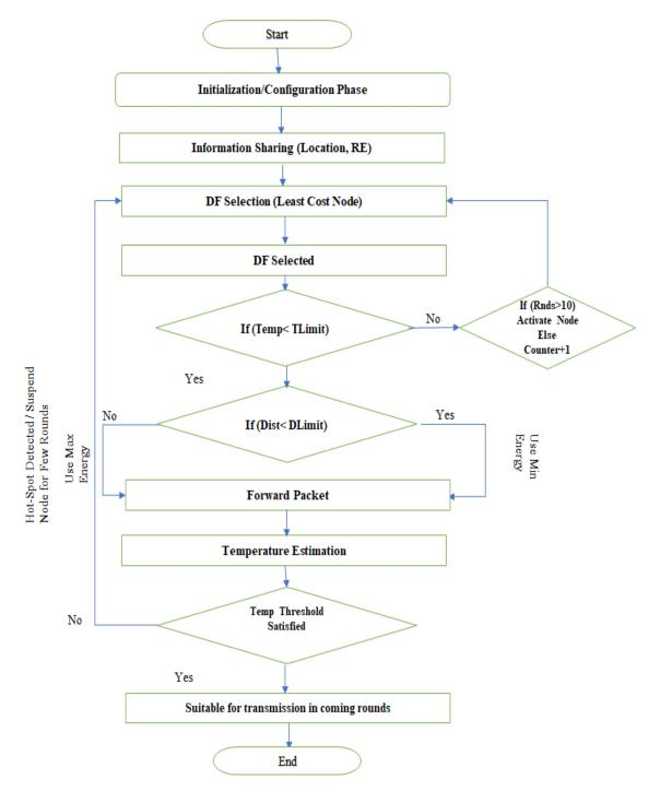
Figure 2. Operational Flow Diagram.
