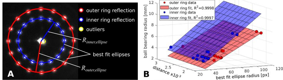
**Figure 2.** (A) Lenstar image of a ball bearing showing the automatically segmented reflective light spots and best fit ellipses for inner and outer ring rings. (B) Surface plots showing the linear correlations between the known radius of curvature of the imaged ball bearings, the radius of the best fit ellipses, and the distance parameter.
