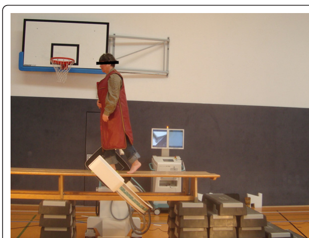
Figure 1 Experimental set-up during data acquisition by dynamic fluoroscopic imaging. The testing person is performing a complete roll-over process of the gait cycle within the measurement field of the flat panel detector which is turned to an oblique position.
