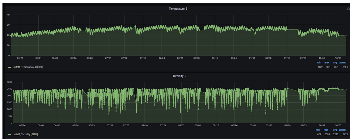
Fig. 10. Temperature and turbidity data collected from June to October 2021, with a sampling rate of 2 min. Data show daily patterns influenced by the repetitive activities in the pond.
