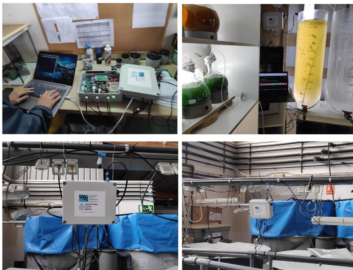
Fig. 9. Deployment of the ADO system in the Aquaculture Center in the Ebre's Delta. Device testing (top-left and right) and nodes installed in final positions (top-right, bottom-left and right).
