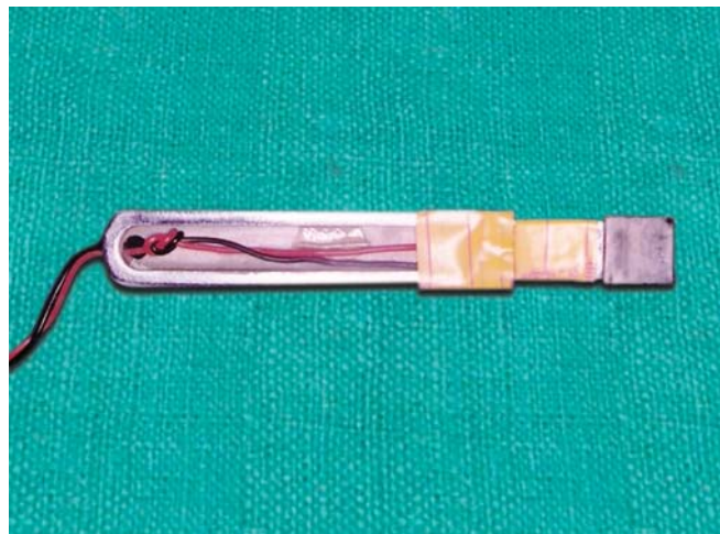
Fig. 2: Parts of metallic fork and sensor
