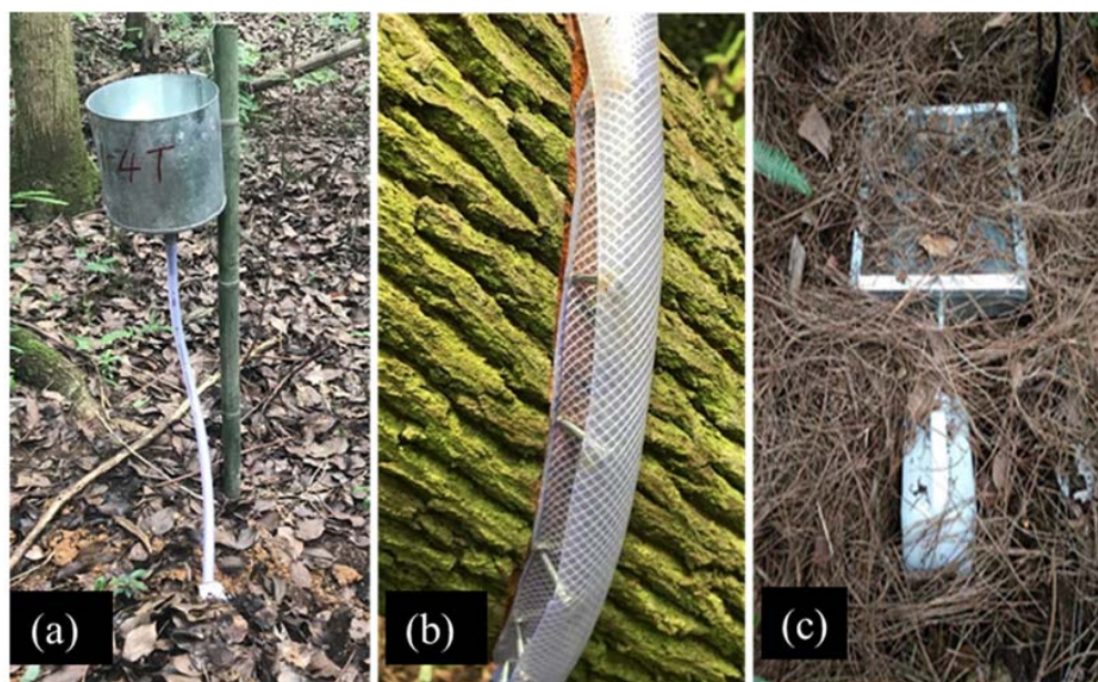
Figure 1. Water sample collectors: (a) throughfall, (b) stemflow, (c) litter leachate.
