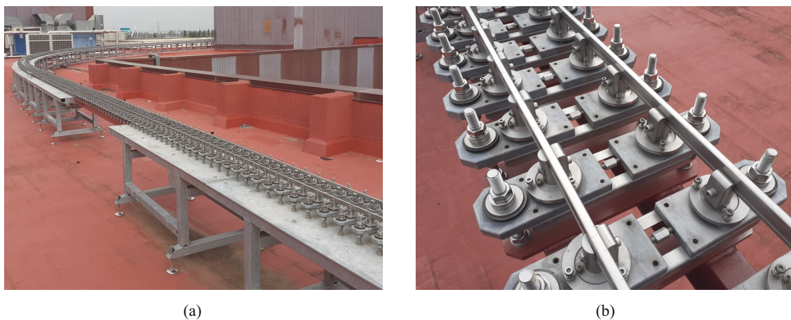
Figure 4. Scaled track assembly (a) and mechanical sleepers (b).
