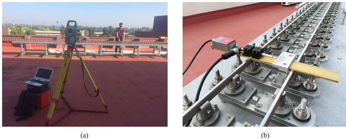
Figure 5. Author measuring the TCL with the robotic total station (a). Track gauge and cant angle measuring device (b).
