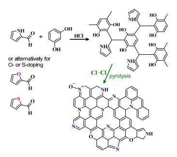
**Figure 1.** Schematic representation of the polycondensation reaction, the cross-linked polymer structure, the utilized heteroaromatic aldehydes, and pyrolysis under chlorine.
