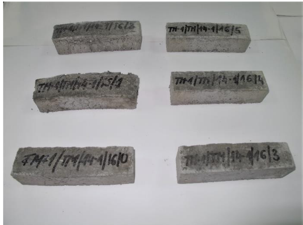
Figure 12. View of TM-1/TM/14-1 repair mortar samples after freeze-thaw cycles according to [19]. Visible deformation, cracks and weight loss of the samples, especially with the following designations: TM-1/TM/14-1/16/0, TM-1/TM/14-1/16/1 and TM-1/TM/14-1/16/2.
