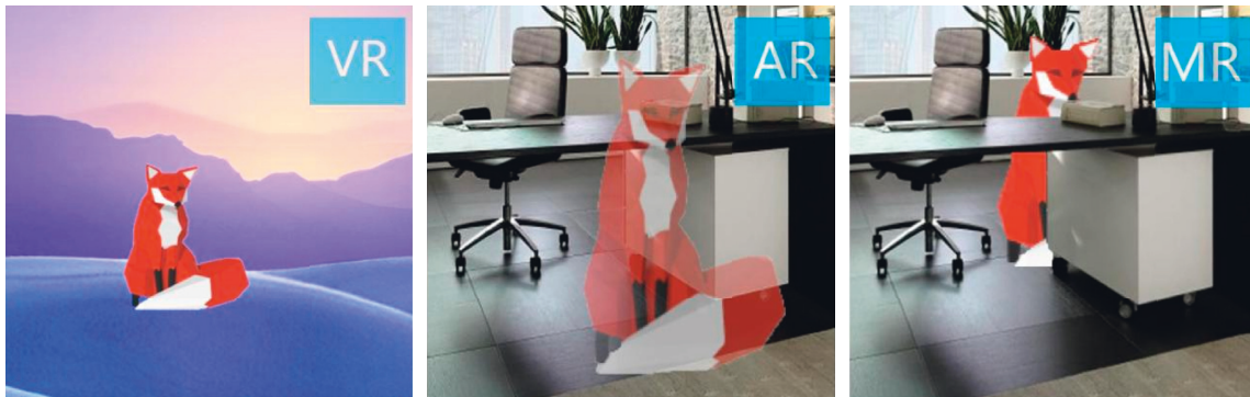
FIGURE 6: Difference between 3 main domains of immersive technology: VR is an artificial world; AR is an object of augmented reality seen on the screen; MR is a 3D object seen as a hologram which is totally controllable.
