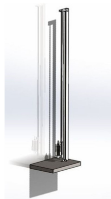
Figure 3. Schematic setup of the test rig for impact toughness measurements.
