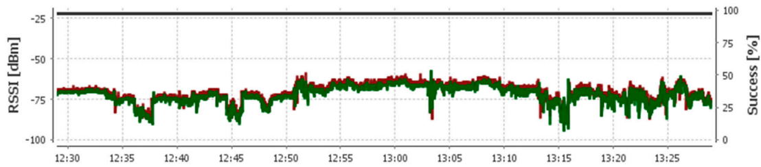
Figure 20. RSSI with interference.
