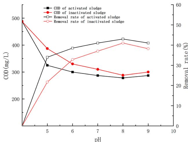
**Figure 4.** Effect of pH on sludge adsorption.
