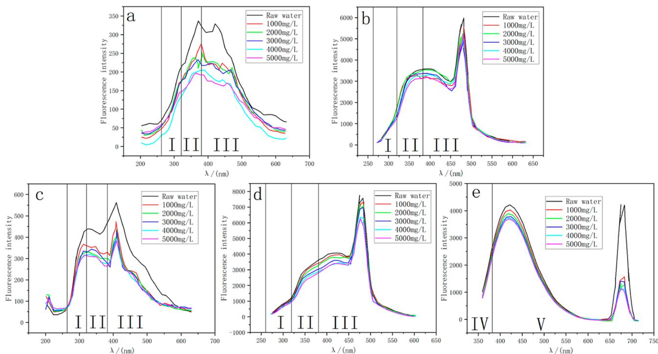
**Figure 3.** Fluorescence scanning spectra of wastewater before and after adsorption and degradation at excitation wavelengths of 200 (a) and 237 nm (b) by activated sludge, and at excitation wavelength of 200 (c), 237 (d), and 340 nm (e) by inactivated sludge.
