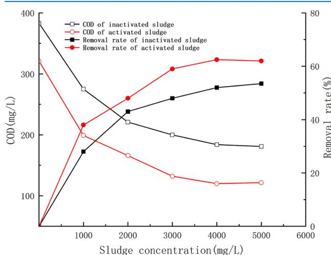
**Figure 2.** Effect of sludge concentration on sludge adsorption.
