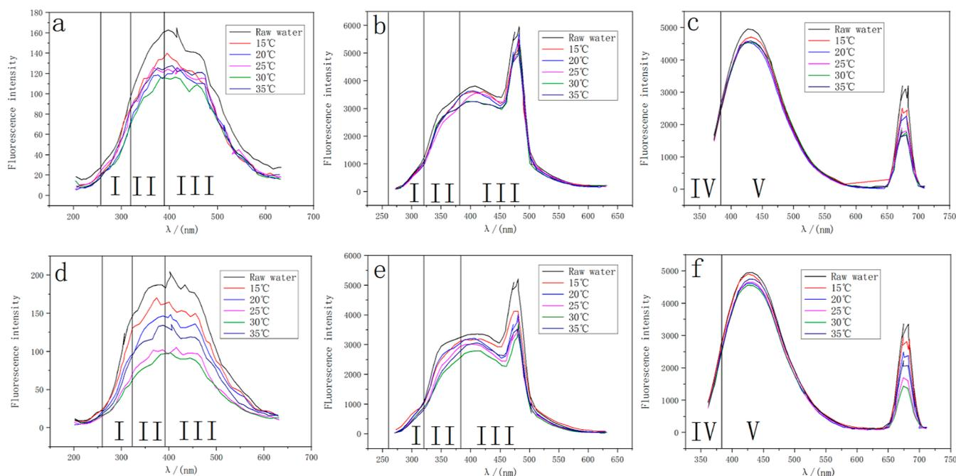
**Figure 7.** Fluorescence scanning spectra of wastewater before and after adsorption and degradation at excitation wavelength of 200 (a), 237 (b), and 340 nm (c) by activated sludge and at excitation wavelength of 200 (d), 237 (e), and 340 nm (f) by inactivated sludge.
