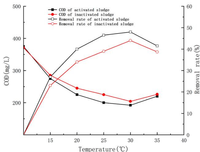
**Figure 6.** Effect of temperature on sludge adsorption.
