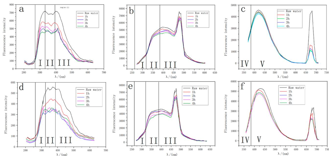
**Figure 1.** Fluorescence scanning spectra of wastewater before and after adsorption and degradation at excitation wavelength of 200 (a), 237 (b), and 340 nm (c) by activated sludge and at excitation wavelength of 200 (d), 237 (e), and 340 nm (f) by inactivated sludge.
