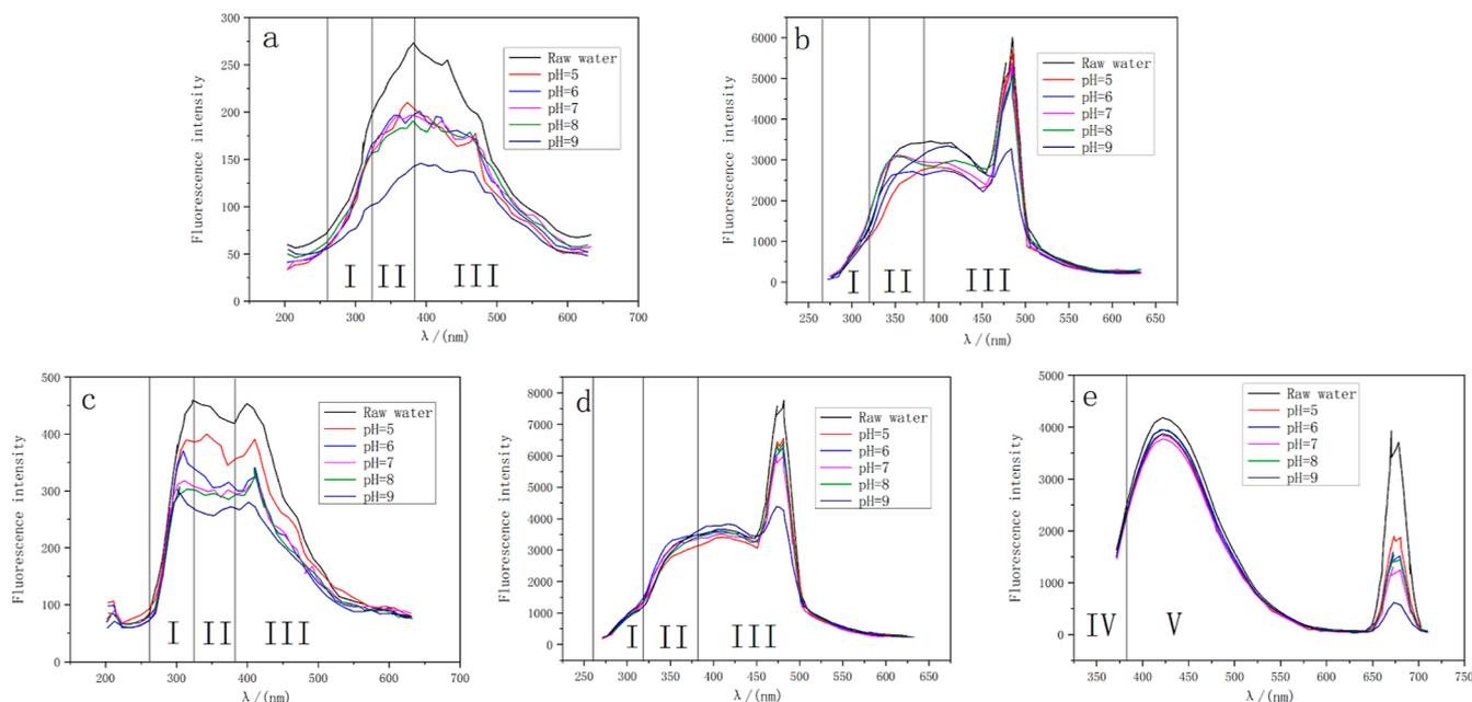
**Figure 5.** Fluorescence scanning spectra of wastewater before and after adsorption and degradation at excitation wavelength of 200 (a) and 237 nm (b) by activated sludge and at excitation wavelengths of 200 (c), 237 (d), and 340 nm (e) by inactivated sludge.
