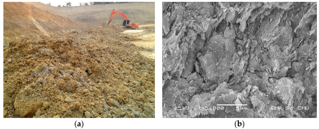
Figure 5. Lateritic soil (a) in overview; (b) microstructure.
