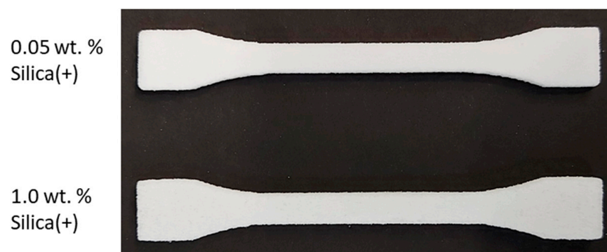
Figure 10. Tensile strength specimens built from PP functionalized with Silica(+).
