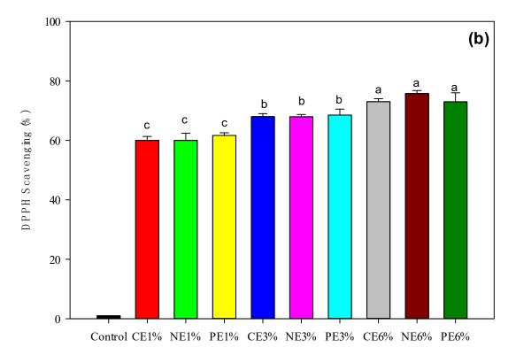
**Figure 3.** Effectiveness of LDPE film treated with cold plasma containing CE-, NE-, and PE-stabilized MFEO. (a) Total phenolic content; (b) antioxidant activity through the DPPH radical scavenging assay. <sup>a–c</sup> The values with different superscripts are significantly different at p < 0.05. The error bars represent the standard deviations (n = 3).
