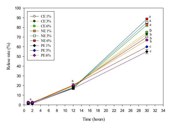
**Figure 5.** Release rate of LDPE film treated with cold plasma containing CE-, NE-, and PE-stabilized MFEO in 95% alcohol. Values with different superscripts are significantly different at p < 0.05. The error bars represent the standard deviation (n = 3).
