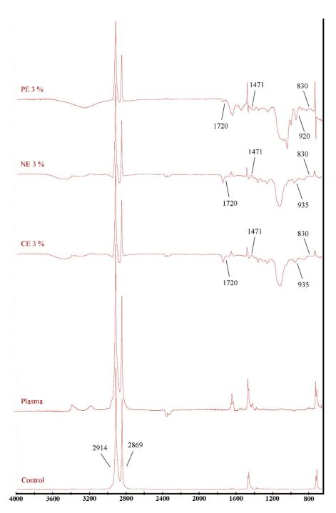
**Figure 1.** ATR–FTIR of LDPE film treated with cold plasma containing CE-, NE-, and PE-stabilized MFEO.
