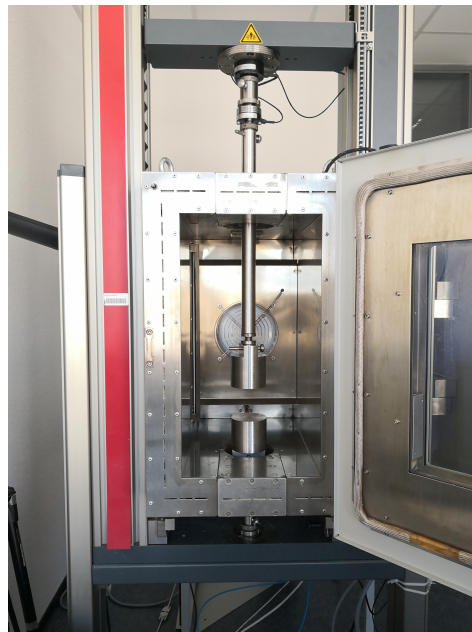
Figure 2. Thermal chamber with the uniaxial compression test setup.
