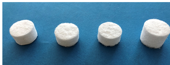
Figure 3. Photograph of the four different aerogel composites based on the following fiber mats. Left to right: FFM, TH, THZ, and FC.
