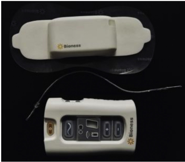
Figure 2. An image of a percutaneous PNS showcases the 3 components of the system: the external pulse transmitter (EPT) and electrode patch, the implanted lead, and the patient programmer. In the top portion of the image is the EPT on top of the electrode patch. Whenever the patient wishes to trigger stimulation for pain relief, they place the electrode patch on their forearm's skin, directly overlying the trajectory of the implanted lead. The EPT is subsequently attached to the electrode patch, delivering neuromuscular electrical field stimulation through the electrode patch to the implanted lead. In the middle portion of the image is one of the leads that were implanted parallel to the patient's left median nerve. In the bottom portion of the image is the patient programmer, which the patient and the medical staff use to adjust the stimulation parameters after implantation. Reprinted with permission (RightsLink License Number 5218290570729) from Ferreira-Dos-Santos et al. 11
