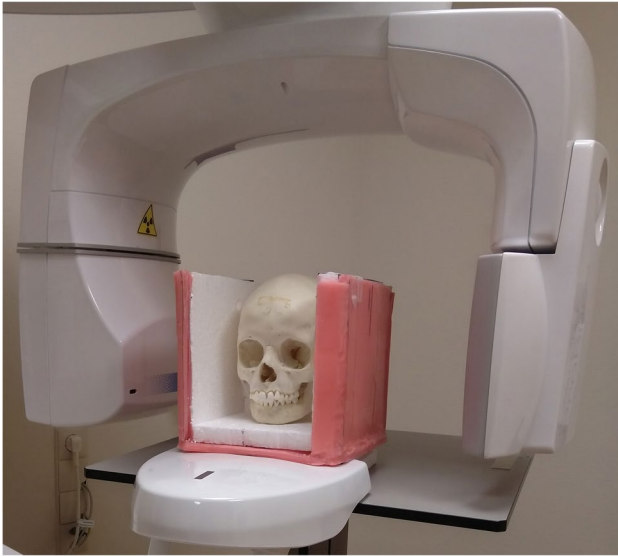
Fig. 1 Dry skull in EPS box with 1-cm utility wax positioned in CBCT machine (front part removed for photo)
