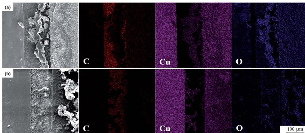
Fig. 5 SEM and elemental mapping images of spacing after 72 h test. (a) Group E1; (b) group E2 (left: cathode plate, right: anode plate).
