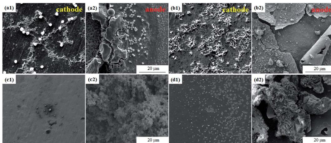
Fig. 6 SEM morphologies of the PCB-Cu exposed in the experimental environment for 24 h (a and c) and 168 h (b and d). (a and b) Group E1; (c and d) group E2.
