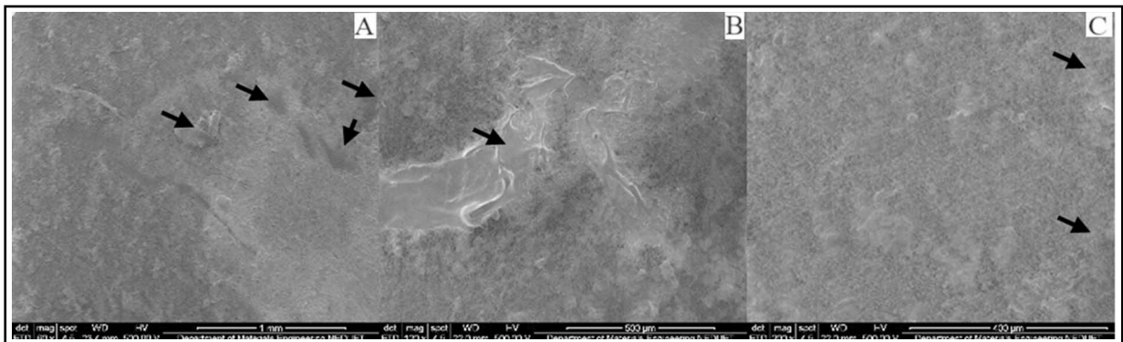
Fig.2: SEM micrographs of nano-filled composite specimen immersed in citric acid at different magnifications.
