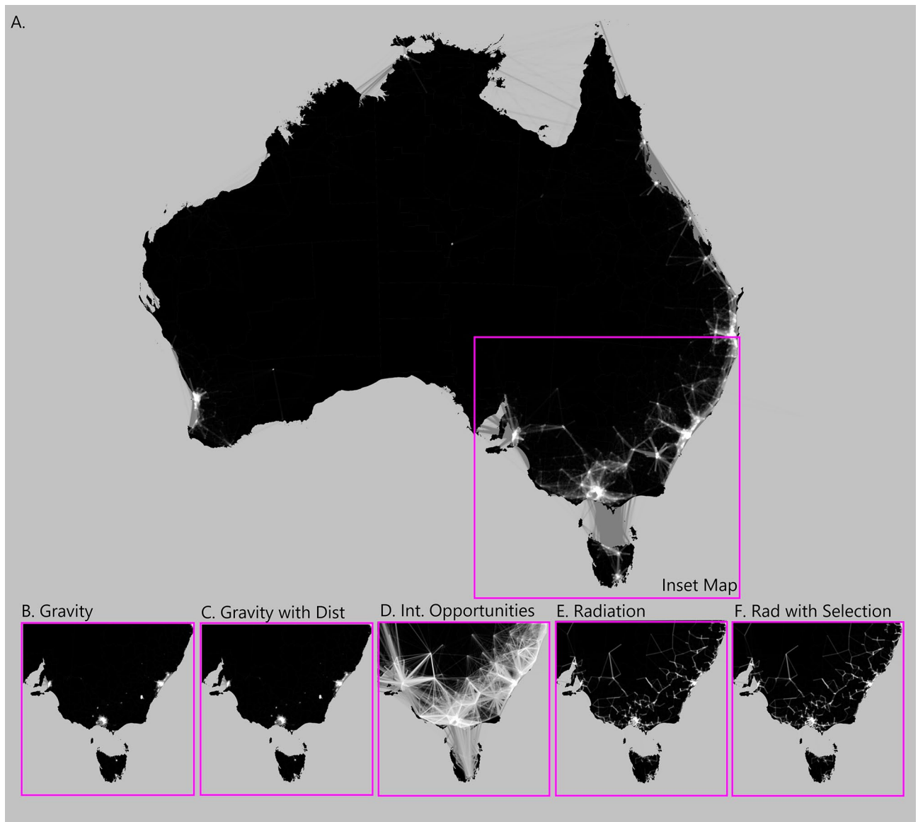
Figure 4. Ensemble model predictions for Australia using ABS census data (A). Inset maps for gravity (B), gravity with distance (C), intervening opportunities (D), radiation (E) and radiation with selection (F) models respectively all trained using ABS data. Movement predictions from each model were scaled to be between 0 and 1 to aid visual comparison. Vivid thick white lines represent high intensity movement, whilst faint thin darker lines represent low intensity movement. The maps in this figure were produced using the R 33 package ggplot2 34 (see Visualisation of predictions section in Methods for further detail). Preview 35 and Paint 3D 36 were used to combine the maps into one image, overlay the squares and add the text.
