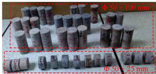
**Figure 21.** The processed rock samples.
