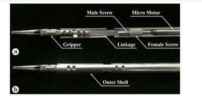
**Fig. 4** Surgical instrument manufactured using aluminum. **a** The surgical instrument without the *upper outer shell*. Actual position of the micro motor, male and female screw, linkage, and the gripper is shown. **b** The surgical instrument with the *upper outer shell*
