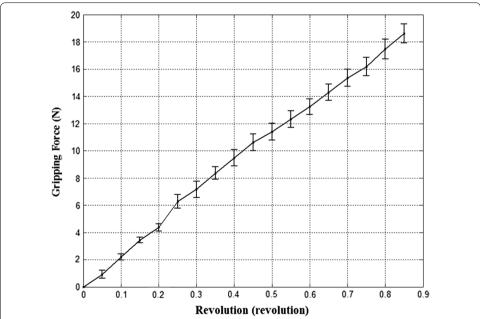
**Fig. 8** Experimental results of gripping force compliant with position of the micro motor. The experiments repeated 10 times and the standard deviation is plotted as *error bar*. The interval of the position of the micro motor was 0.05 revs
