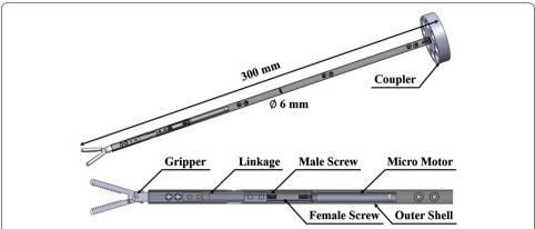
**Fig. 3** Design of the proposed surgical instrument. The gripping motion is achieved by converting the micro motor's rotation motion into linear motion by male and female screw and linking the gripper with the female screw through the linkage. The length and the diameter of the surgical instrument is designed as 300 mm and 6 mm, respectively
