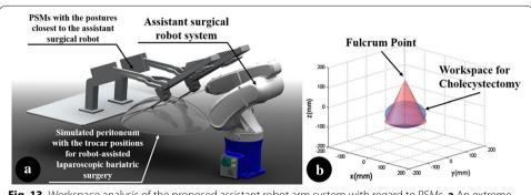
**Fig. 13** Workspace analysis of the proposed assistant robot arm system with regard to PSMs. **a** An extreme condition to the assistant robot arm system's workspace. **b** Calculated workspace in the extreme condition
