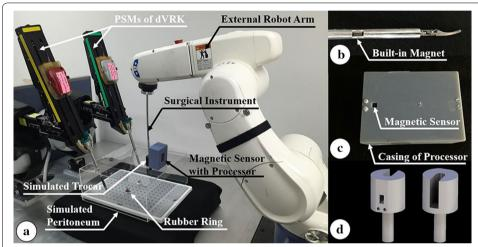
**Fig. 11** Setup for the in vitro test of semi-automatic resected object removal. **a** Overall system setup. **b** Built-in magnet of the surgical instrument to generate magnetic field. **c** Magnetic sensor with its controller board within the special housing. **d** Developed simulated trocar used in the in vitro test
