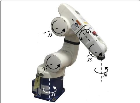
**Fig. 5** Joint information of the 6-degrees of freedom (DOFs) external robot arm. The fulcrum point motion and the translational motion of the surgical instrument are achieved by complex combination from *J1* to *J5*. The surgical instrument's rolling motion is achieved by *J6*
