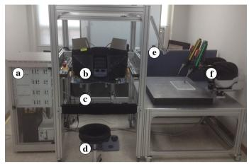
**Fig. 2** Overall system of the da Vinci research kit (dVRK). **a** Controllers. **b** Stereo viewer. **c** Master tool manipulators (MTMs). **d** Foot pedal. **e** Two webcams for providing images. **f** Patient side manipulators (PSMs). dVRK is used as operation surgical robot system in this research
