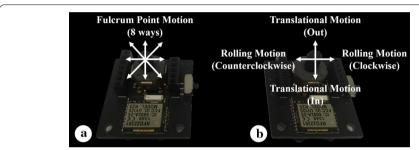
Fig. 7 Mapping information between the NMI and the surgical instrument. a Left NMI. b Right NMI
