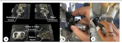
Fig. 6 Developed novel master interface (NMI). a Front and back side of the NMI. b The NMI attached on the MTM of the dVRK system using the special holder. c Usage of the index finger to operate finger clutch and the NMI
