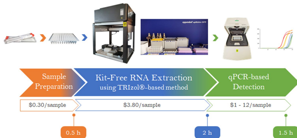
Figure 1. Scalable high-throughput kit-free RNA extraction workflow. Biological samples are manually transferred into a 96-well PCR plate and total RNA extraction was carried out by automated liquid handlers using a modified TRIzol-based method. Manual intervention is required for plate centrifugation. Viral diagnostic analyses is performed on extracted RNA via qPCR-based detection. A complete run of 96 samples takes 4 h. The cost (USD) per sample was calculated based on actual local prices and includes laboratory consumables such as tips and reagents but excludes the cost of instruments.
