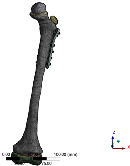
Fig. 4 Mesh model after assembly and internal fixation.
