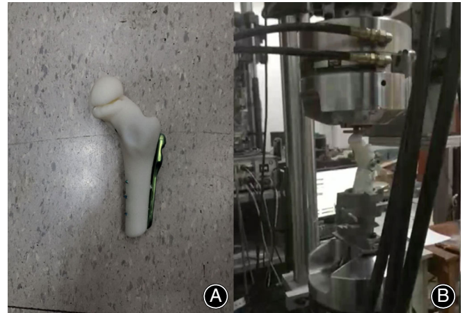
Fig. 6 The picture shows the pressure test and the cracking part of the model.
