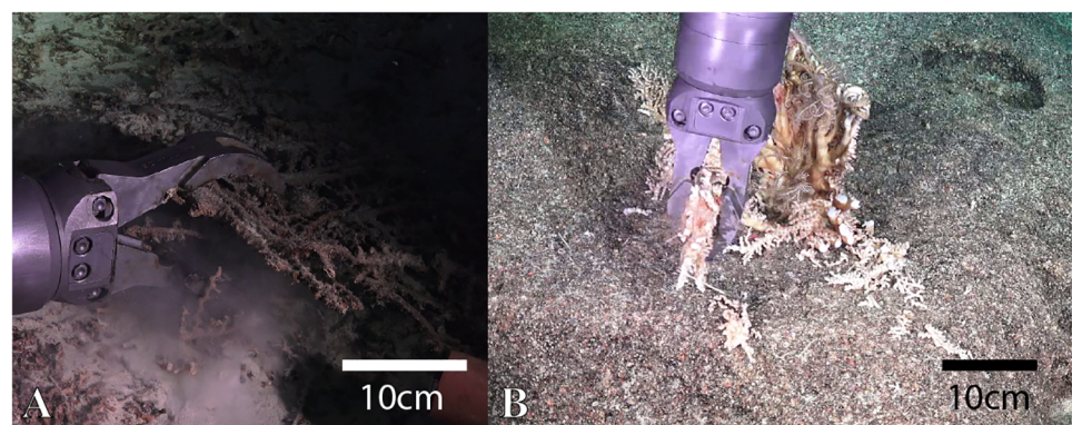
Fig 11. Challenges when grasping brittle specimens with hard bodied manipulators. A: Coral rubble (depth: 616m, S1 Video). B: Enallopsammia sp. coral (depth: 434m).
