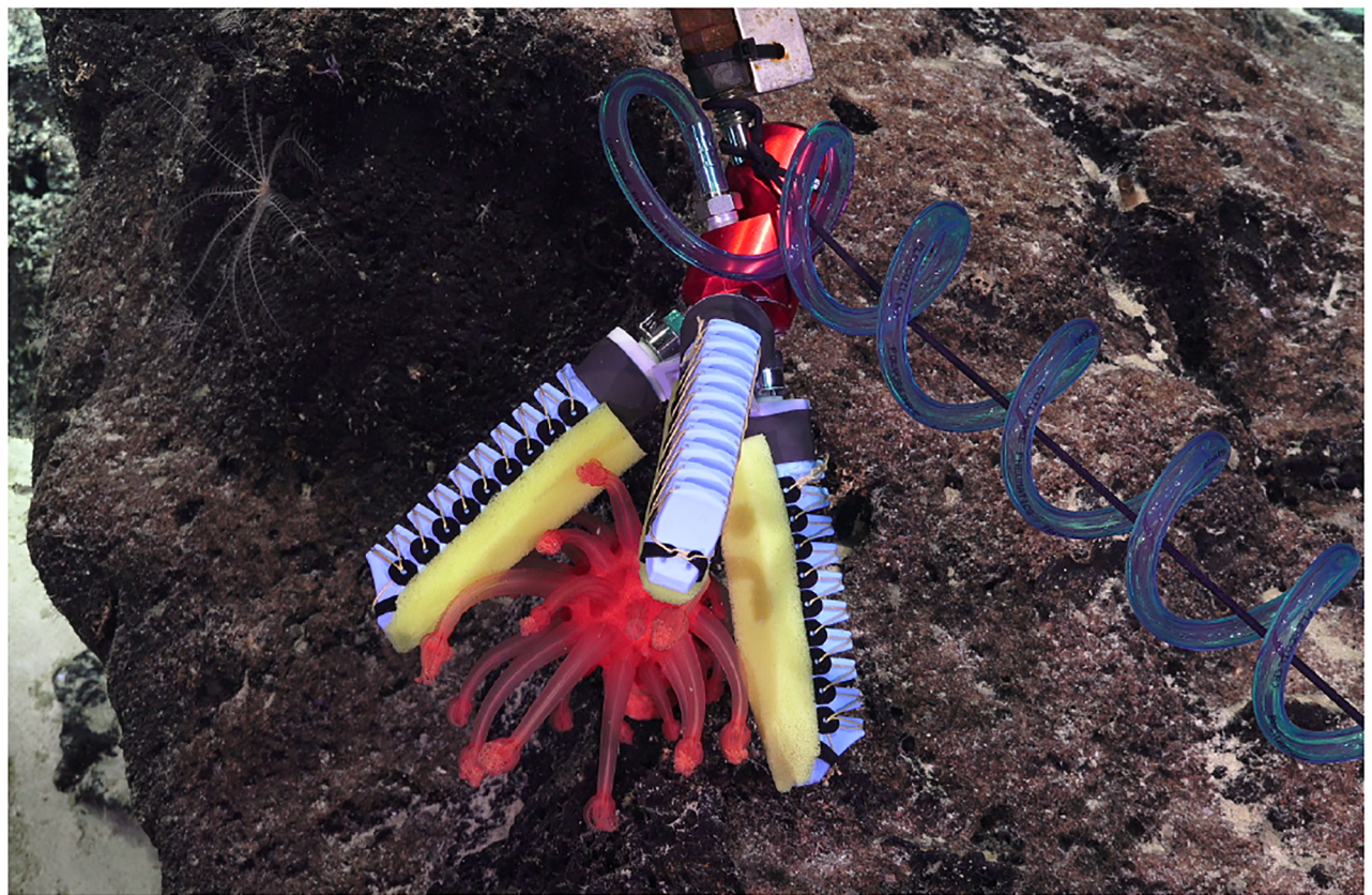
Fig 13. Difficulties in grasping. Example of orienting the manipulator horizontally or perpendicularly from a deep-sea mushroom coral ( Anthomastus sp., depth: 1282m).
