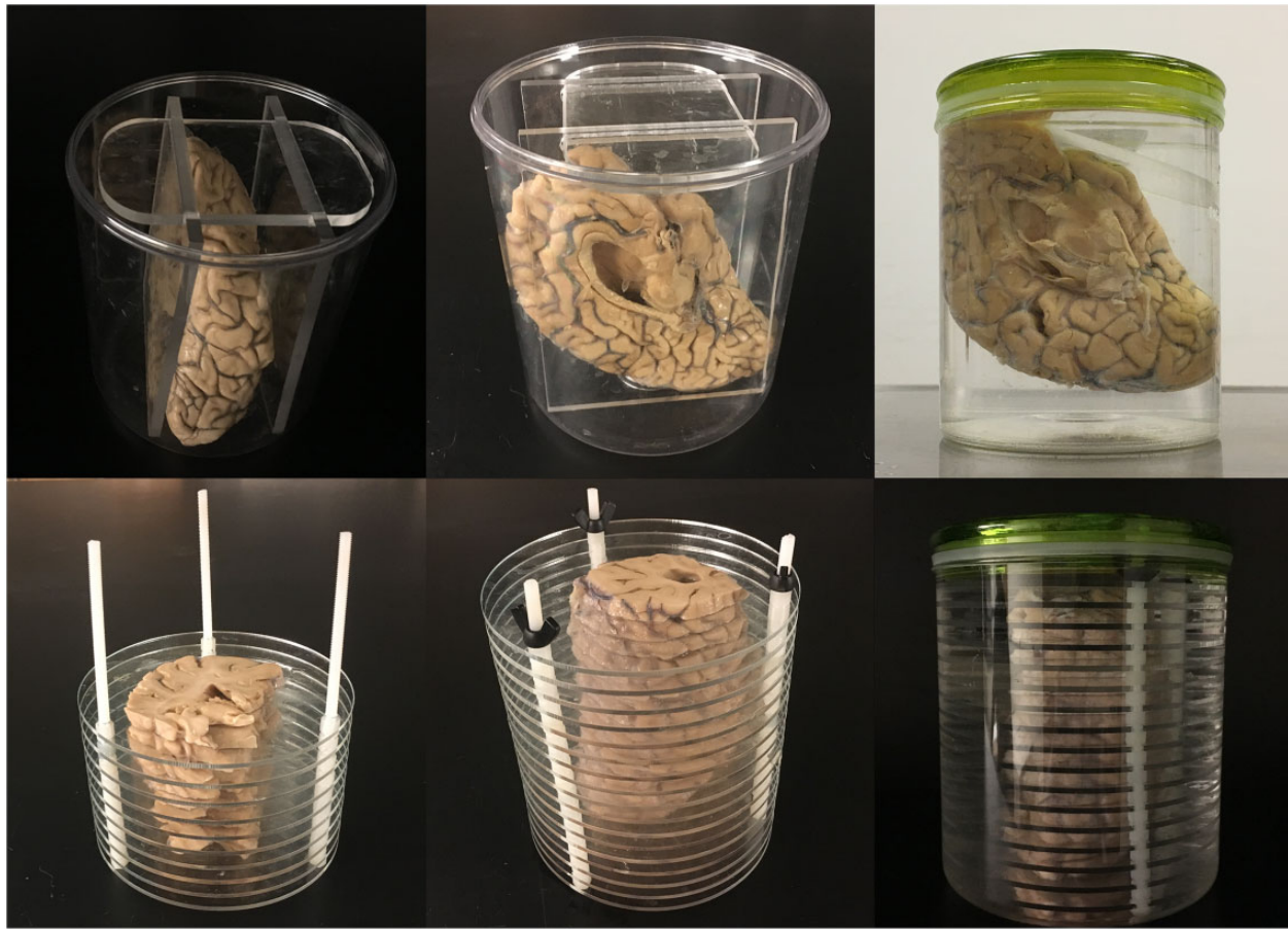
Figure 1. Whole hemisphere sample preparation for MRI (top) and sliced hemispheres (bottom). Samples are submerged in Fluorinert inside a vacuum sealed container (The ConBrainer). Sample orientation is maintained with interlocking plastic struts (whole hemisphere) or plastic disks with 6-mm spacers (slices.).
