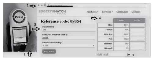
Fig. 2. Four steps of obtaining the recipe for a specimen (Specimen C25-1) using e-skin system (1) Measuring the specimen using spectrocolorometer and obtaining its color code (2) Finding E-skin system's on-line calculator (3) Entering the color code into calculator (4) Obtaining the recipe for a desired amount of silicone.
