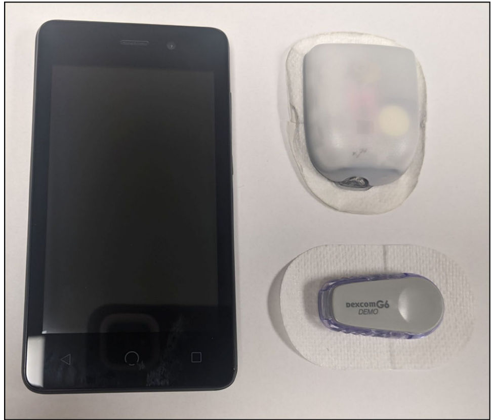
Fig. 4 Omnipod patch pump (top right) with personal diabetes manager (left) and Dexcom G6 continuous glucose monitor (bottom right)
