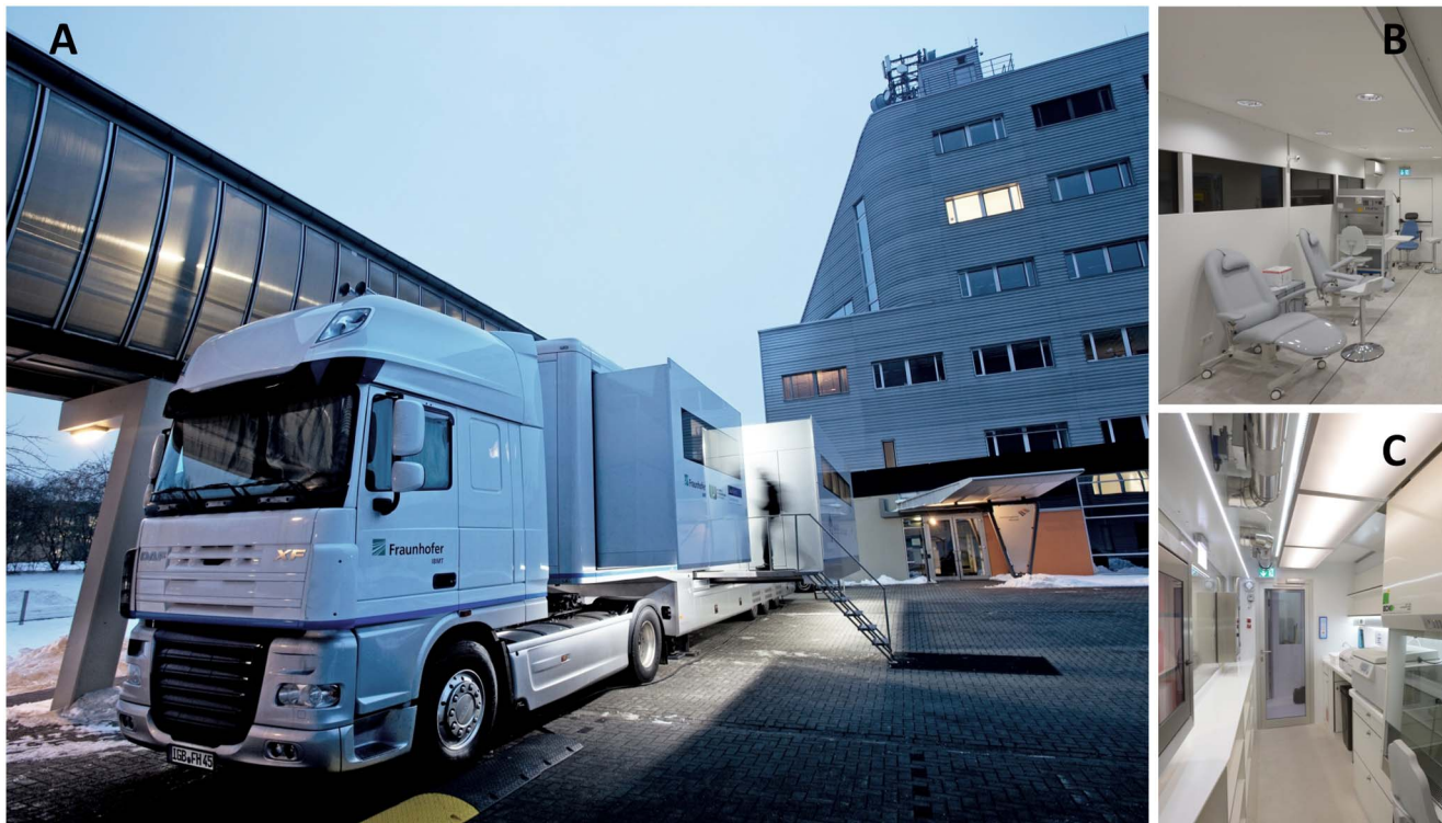
Figure 2. Mobile epiLab at first mission. A: The expandable unit. B: View to the examination room. C: BSL-2 area in the mobile epiLab with urine processing area (background) and blood processing area (foreground). doi:10.1371/journal.pone.0105401.g002
