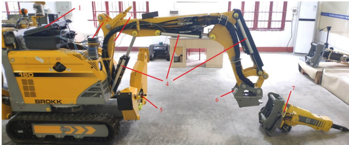
Figure 9. Attachment changing experimental conditions. (1) Nvidia Jetson TX2 and sensors serial communication module, (2) wireless router, (3) inclinometer, (4) displacement sensors, (5) industrial camera, (6) error compensation reference tag, (7) positioning tag of attachment.
