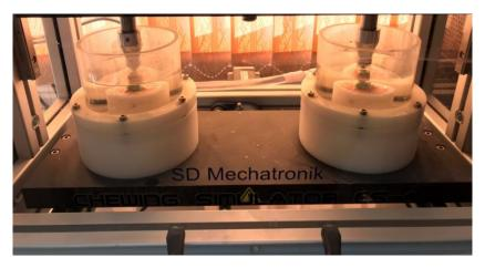
Figure 1: Studied specimens in chewing simulator machine
