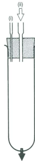
Figure 4.2. Apparatus for harvesting sucrose gradients (from Minor 1985).
