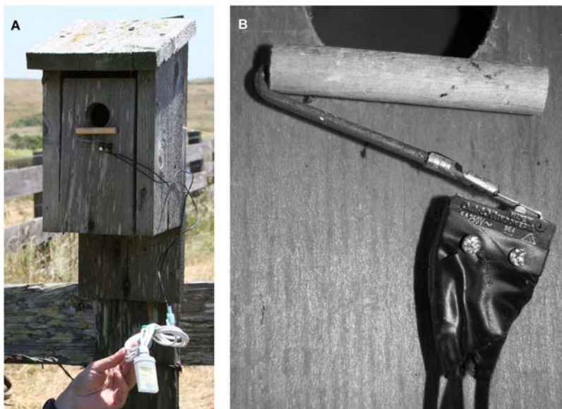
Figure 1. Nest box with Automatic Perch Recorder attached. The apparatus consists of a dowel-perch attached to a microswitch mounted at the cavity entrance (close-up in panel B), which is in turn connected to an event recording data logger—visible in bottom right of panel A. doi:10.1371/journal.pone.0004111.g001
