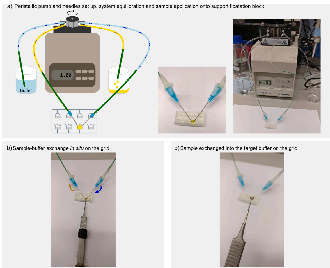
Fig. 3. Prefixation protocol and buffer exchange in situ with the support floatation block. a) Diagram showing the preparation of PreFix gradients and images of gradients produced in the laboratory. The gradient shown has been tinted using food colouring to visualise the different regions. b) Diagram and images showing the buffer exchange setup using the peristaltic pump and the support floatation block. c) Illustration of buffer exchange on a grid using the support floatation block. The peristaltic pump works in opposition to itself to move the wash buffer through the well at a constant rate. Yellow food colouring has been used to visualise the exchange process, which takes only 10–30 s, even for viscous samples. d) Picture of a grid exchanged into the target buffer. (For interpretation of the references to colour in this figure legend, the reader is referred to the web version of this article.)
