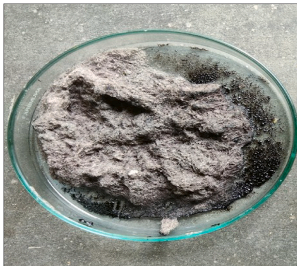
Fig. 1. Microcrystalline Cellulose Powder obtained after 12 h of sonication and 48 h of lyophilization.
