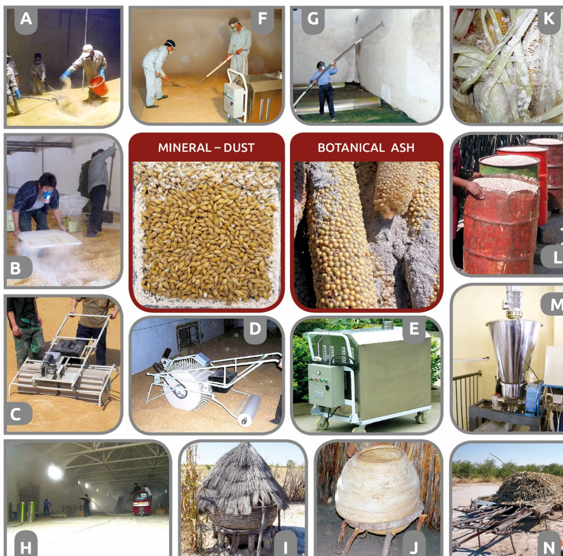
Figure 6. (A,B) Various types of manual applications of inert dusts for surface and subsurface grain treatment in horizontal stores; (C,D) two types of motorized blenders for surface and subsurface grain treatment in horizontal stores (ASAG-Beijing);
