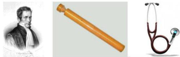
Fig. 1. 1a: Doctor René-Théophile-Hyacinthe Laennec, inventor of the stethoscope. 1b: The stethoscope is a system of transmission and amplification of sound by resonance. Its principle is rather simple. Using a specific interface (diaphragm or bell), a sound is picked up and then transmitted over a small distance to the user's ears. Traditionally, the sound is transmitted in an aerial way via a conduit. 1c: The latest generation of stethoscopes is electronic and uses a microphone system and speakers to restore sounds ( adapted from the chapter: Advances and Perspectives in the Field of Auscultation, with a Special Focus on the Contribution of New Intelligent Communicating Stethoscope Systems in Clinical Practice, in Teaching and Telemedicine. InTech 2012. http://dx.doi.org/10.5772/48402 ).
