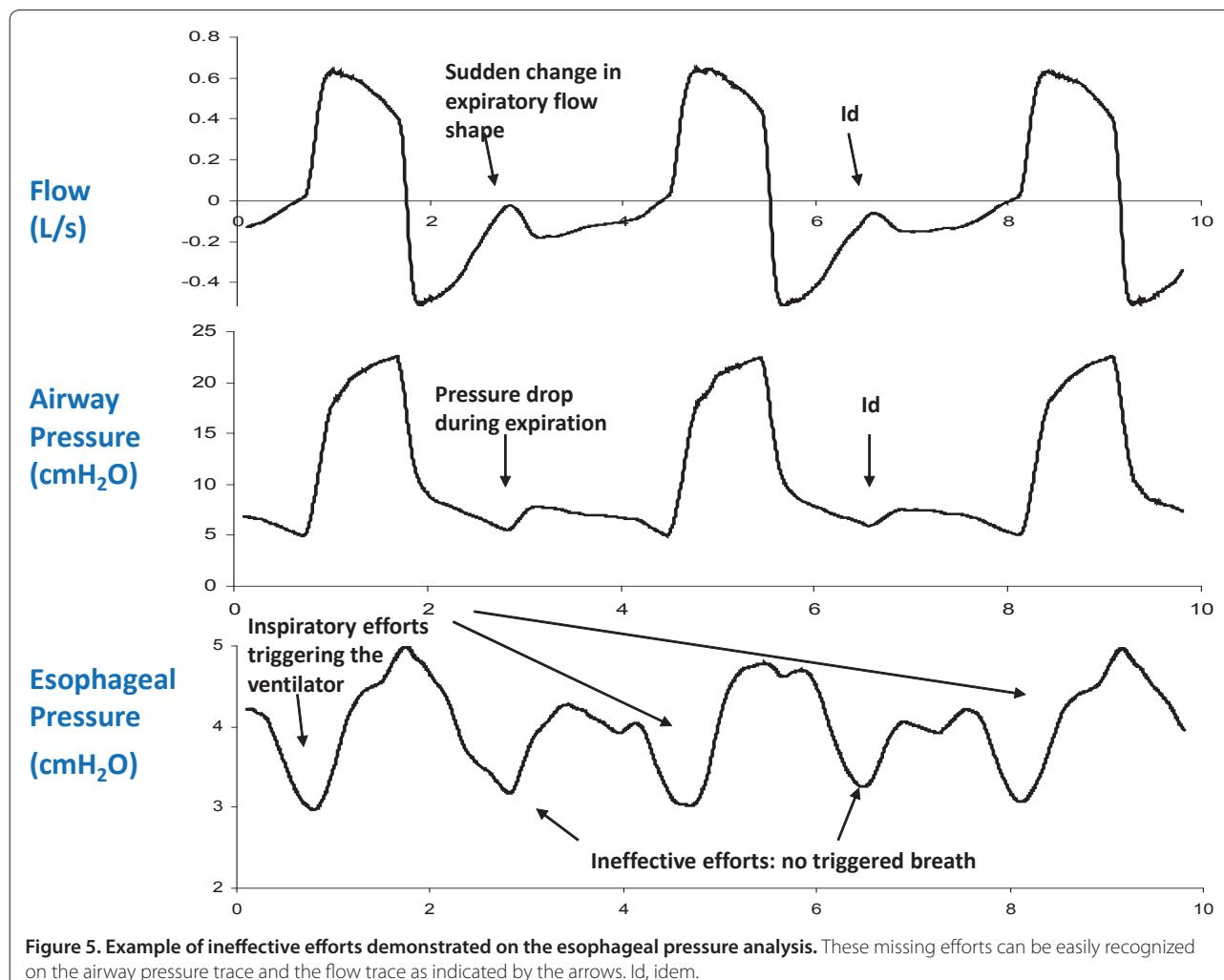
**Figure 5.** Example of ineffective efforts demonstrated on the esophageal pressure analysis. These missing efforts can be easily recognized on the airway pressure trace and the flow trace as indicated by the arrows. Id, idem.
