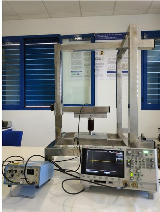
**Figure 1.** Photograph of the measurement set-up for the determination of ultrasound parameters.
