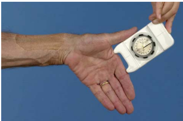
Fig. 1 Inclinometer used for measuring of movements
