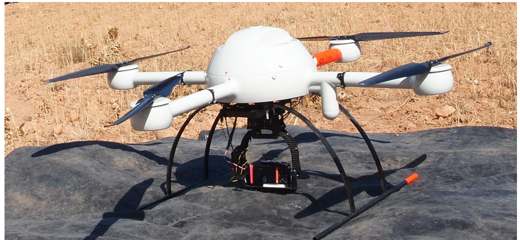
Fig 2. UAV utilizing a mounted SONY \alpha ILCE-5100L sensor + E 20 mm F2.8 lens.
