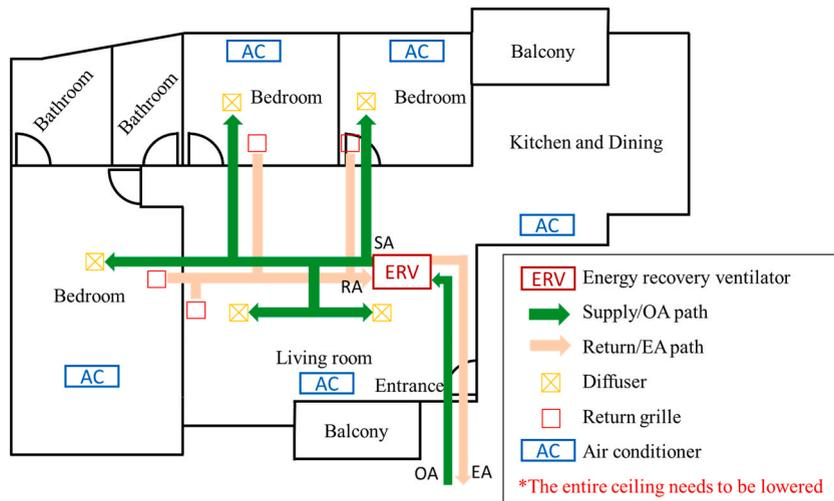
Fig. 2. Installation scheme of a typical ERV for the three-bedroom condo.
