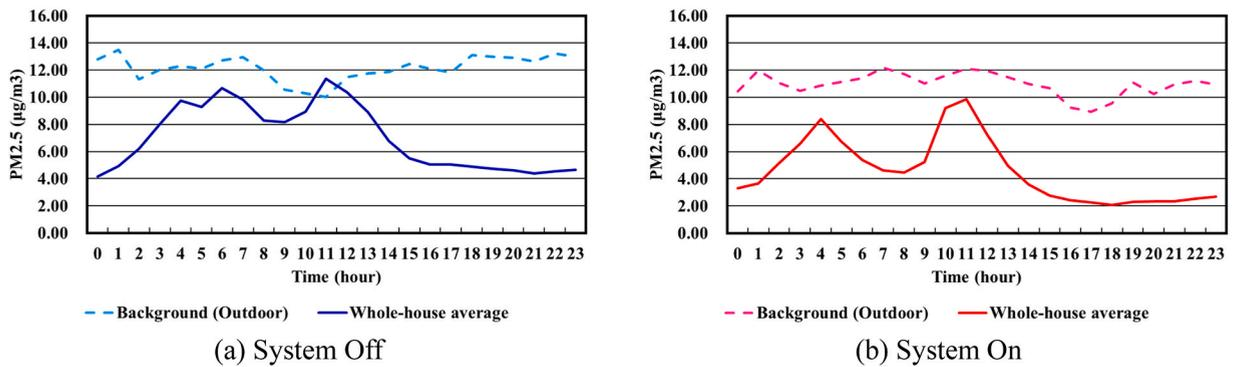
Fig. 9. The hourly background (outdoor) versus whole-house average PM<sub>2.5</sub> concentration in the CR-ERV system on and off periods. (a) System Off, (b) System On.
