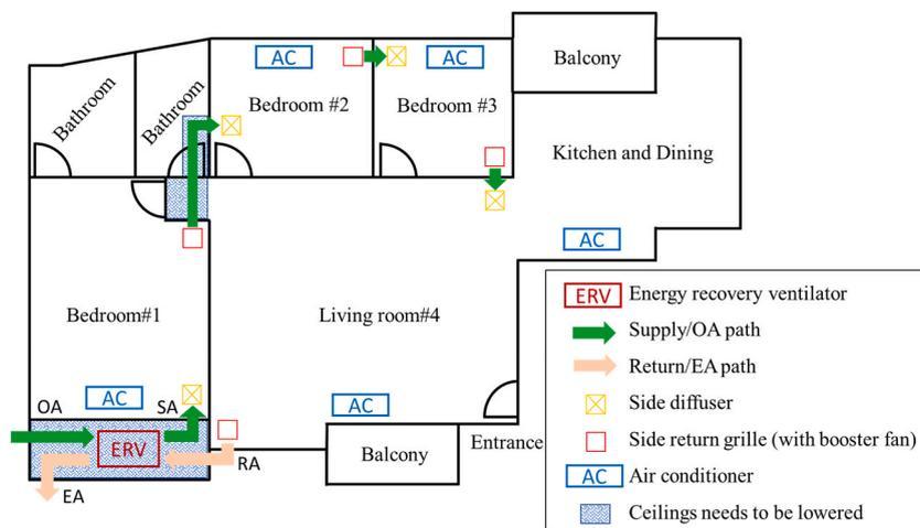
Fig. 3. Installation scheme of a CR-ERV for the three-bedroom condo.
