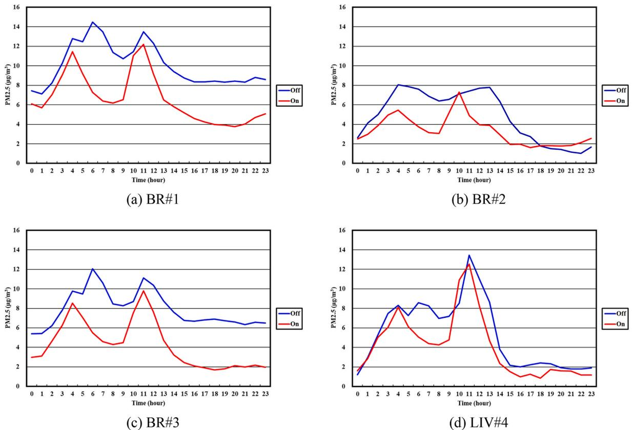
**Fig. 8.** The hourly average PM<sub>2.5</sub> concentration difference in each monitored zones between the CR-ERV system on and off periods. (a) BR#1, (b) BR#2, (c) BR#3, (d) LIV#4.
