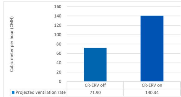
**Fig. 10.** The projected whole-house average ventilation rate during the CR-ERV system on and off periods (from 4:00 to 9:00 a.m.).
