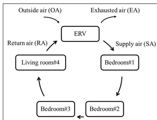
Fig. 4. The airflow path of the CR-ERV system.
