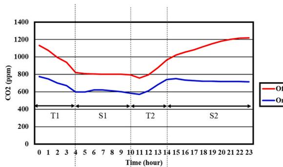
**Fig. 11.** The 24-h variation of whole-house average CO<sub>2</sub> concentration during the CR-ERV system on and off periods.
