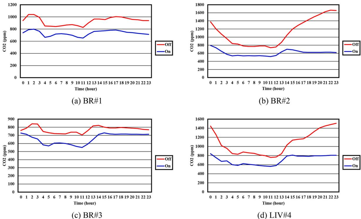
**Fig. 6.** The hourly average CO<sub>2</sub> concentration difference in each monitored zones between the CR-ERV system on and off periods. (a) BR#1, (b) BR#2, (c) BR#3, (d) LIV#4.
