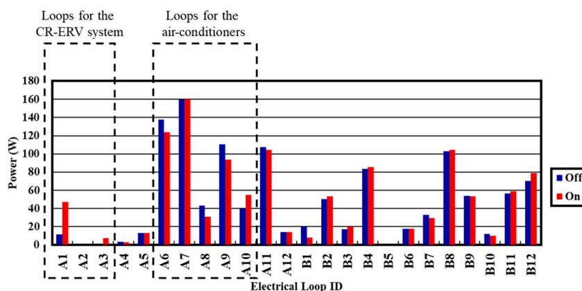
Fig. 13. The average power consumption of each electrical loop during the CR-ERV system on and off periods.
