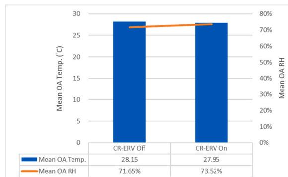
**Fig. 12.** The comparison of mean outdoor temperature and relative humidity during the CR-ERV system on and off periods.
