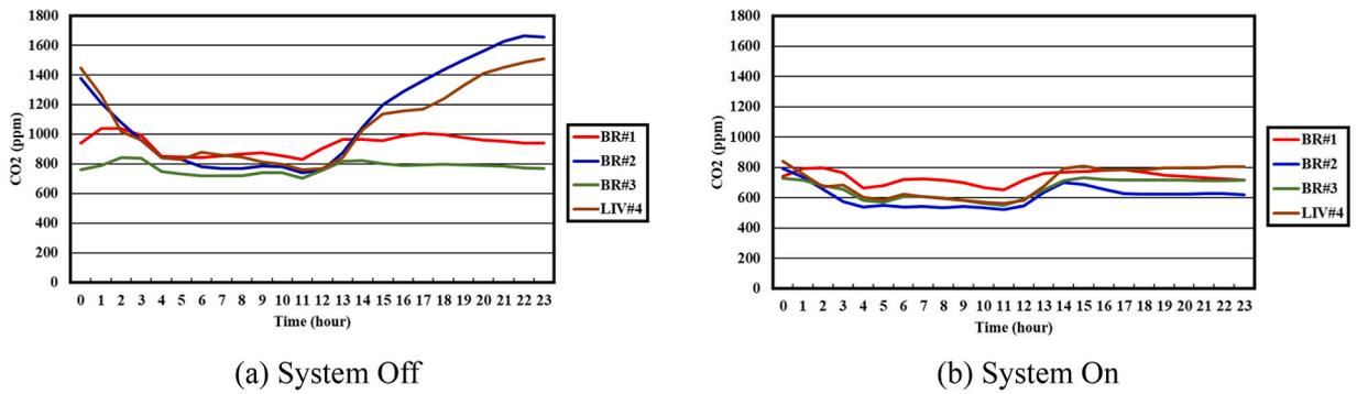
**Fig. 7.** The hourly average CO<sub>2</sub> concentration difference in each monitored zones between the CR-ERV system on and off periods. (a) System Off, (b) System On.
