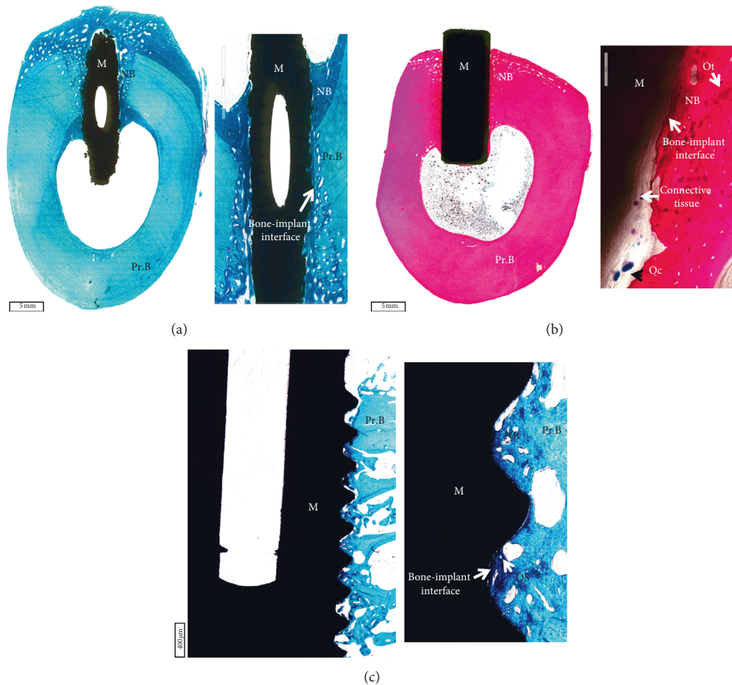
FIGURE 1: (a) Sheep tibial diaphysis six months after a roughened titanium alloy implantation. Toluidine Blue and Fast Green stain: in black, the material; in light green, the preexisting bone; in dark green, the newly formed bone. Left: magnification 1x; right: magnification 30x. (b) Sheep tibial diaphysis three months after a sandblasted titanium implantation. Stevenel's blue and picrofuchsin stain: in black, the material; in fuchsia, the bone; in blue, the cells. Left: magnification 1x; right: magnification 30x. (c) Sheep iliac crest three months after a titanium screw implantation. Toluidine Blue and Fast Green stain: in black, the material; in light green, the preexisting bone; in dark green, the newly formed bone. Left: magnification 10x; right: magnification 30x. M: material; NB: new bone; Pr.B: preexisting bone; Ot: osteocytes; Oc: osteoclasts; OS: osteoid tissue.
